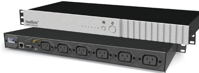
A discreet 1U (44.5mm) high rack width component, offering full system control of connected electronics through RS232, LAN, Bluetooth and over WiFi with a Smartphone App. Alpha features six C14 IEC output sockets along with RS232 via traditional and USB ports, LAN Ethernet port for WiFi control and antenna supporting Bluetooth. Alpha protects connected equipment up to 40000A. Input power is via standard IEC C15/16 connection.
